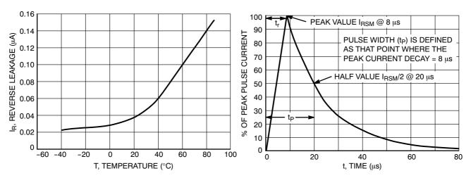
Figure 3. Reverse Leakage versus Temperature
