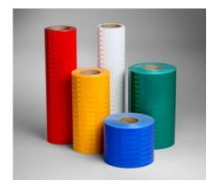
3M™ Engineer Grade Prismatic Reflective Sheeting Series 3430 meets ASTM D4956 Type I and is a non-metalized, microprismatic lens reflective sheeting designed for production of non-critical traffic control signs, work zone devices and delineators that are exposed vertically in service.
