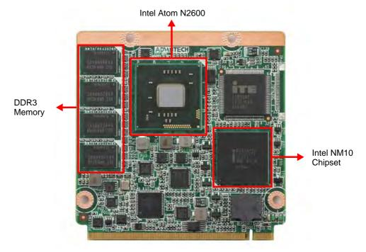
Figure 2.1 Board Chip Placement - Front
