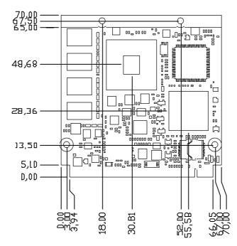
Figure 2.3 Board Mechanical Drawing - Front
