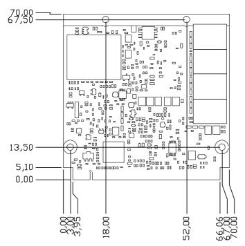
Figure 2.4 Board Mechanical Drawing - Back
