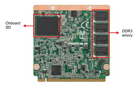
Figure 2.2 Board Chip Placement - Back
