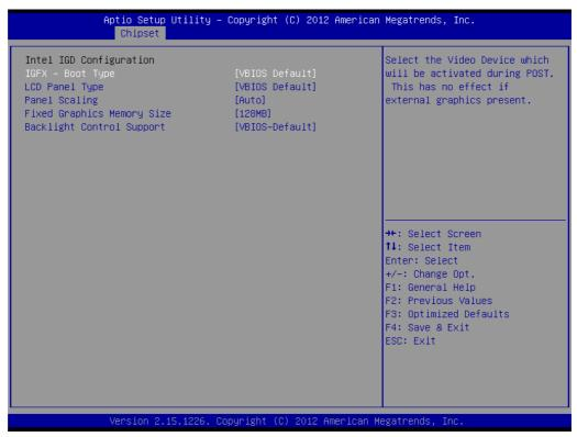
Figure 3.16 Intel IGD Configuration
