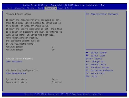
**Figure 3.23 Password Configuration**
