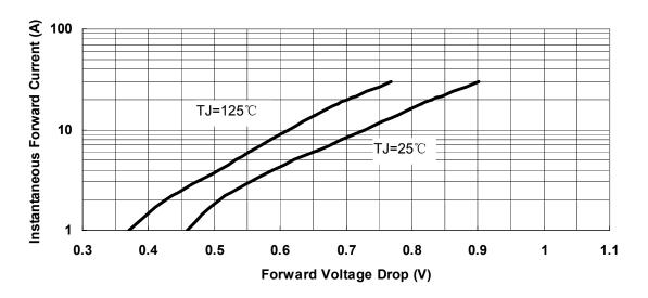
Fig.3-Typical Instantaneous Forward Voltage Characteristics
