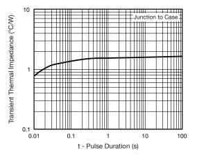
Fig. 6 - Typical Transient Thermal Impedance
