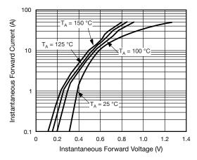
Fig. 3 - Typical Instantaneous Forward Characteristics
