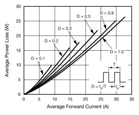
Fig. 2 - Forward Power Loss Characteristics
