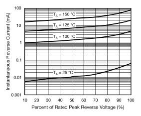
Fig. 4 - Typical Reverse Characteristics
