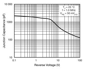
Fig. 5 - Typical Junction Capacitance
