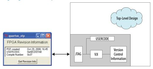
A Tcl script creates and updates the verilog file containing the hardcoded version control information every time the project goes through a full compile. The Tcl script is executed automatically by adding the following assignment to the project's **.qsf** file.
