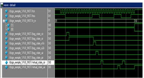
The figure below shows the inputs and outputs of the Virtual JTAG IP core during a typical DR scan shift operation.
