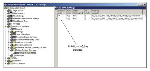
These unique IDs are necessary for the Intel Quartus Prime Tcl API to properly address each instance of the IP core.
