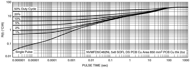
Figure 13. Thermal Characteristics
