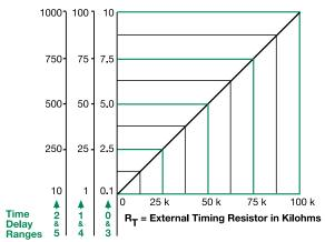
This chart applies to externally adjustable part numbers. The time delay is adjustable over the time delay range selected by varying the resistance across the  $R_{\mathsf{T}}$  terminals; as the resistance increases the tie delay increases
