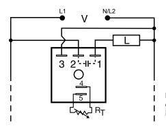
$R_{\scriptscriptstyle T}$  is used when external adjustment is ordered.
