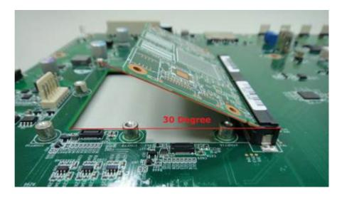
2. Press down the module board and make sure the 4 screw holes are aligned with the carrier board and adjust the 4 screws clockwise to fix them in place
