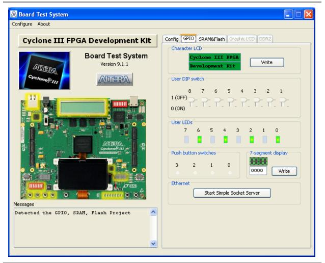
The following sections describe the controls on the GPIO tab.
