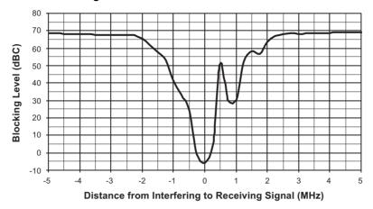
Figure 2-8. Wide-band 3-dB Blocking Characteristic at 315MHz
