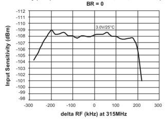
Input Sensitivity (dBm) at BER < 1e-3, ATA8201, FSK, 2.4Kbits/s (Manchester),
