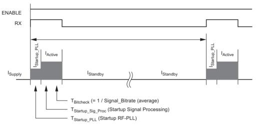
In an industrial or aftermarket RKE and TPM system, the average chip current in Polling mode, I<sub>Polling</sub>, is an important parameter. The polling period must be controlled by the connected microcontroller via the pins ENABLE and RX. The polling current can be calculated as follows:
