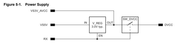
The supply voltage range of the Atmel® ATA8201/ATA8202 is 2.7V to 3.3V or 4.5V to 5.5V.
