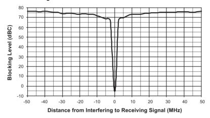
Table 2-8 shows the blocking performance measured relative to -102dBm for some frequencies. Note that sometimes the blocking is measured relative to the sensitivity level 104dBm (denoted dBS), instead of the carrier -102dBm (denoted dBC).
