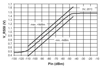
As can be seen in Figure 2-9 on page 12, for single devices there is a variance over temperature and supply voltage range of ±3dB. The total variance over production, temperature, and supply voltage range is ±9dB.
