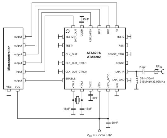
Note: Paddle (backplane) must be connected to GND
