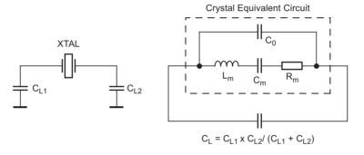
With C<sub>m</sub> ≤ 10fF, C<sub>0</sub> ≥ 1.0pF, C<sub>LN</sub> = 9pF and C<sub>L1,2</sub> = 16pF ±1%, the pulling amounts to P ≤ ±1ppm.
