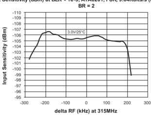
Input Sensitivity (dBm) at BER < 1e-3, ATA8201, FSK, 9.64Kbits/s (Manchester),
