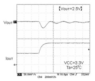
Fig. 17 Transient response Io=250→500mA(10µs)
