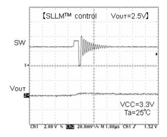
Fig.14 SW waveform Io=10mA
