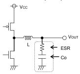
Fig.29 Output capacitor
