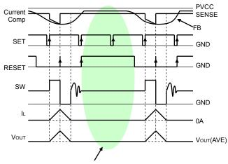
Not switching Fig.21 SLLM<sup>TM</sup> switching timing chart
