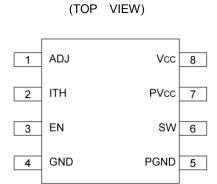
Fig.2 Pin Configuration
