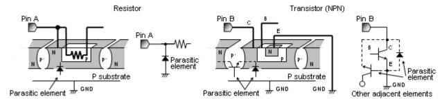
Fig.37 Simplified structure of monorisic IC
