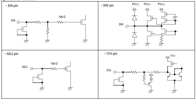
Fig.36 I/O equivalence circuit
