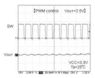
Fig.15 SW waveform Io=500mA
