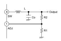
Fig.34 Determination of output voltage
