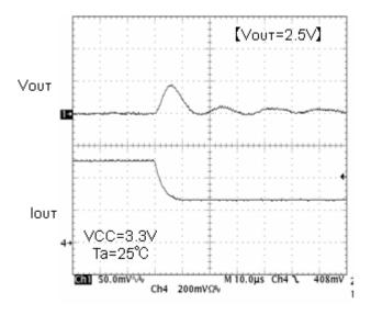
Fig.18 Transient response Io=500→250mA(10µs)
