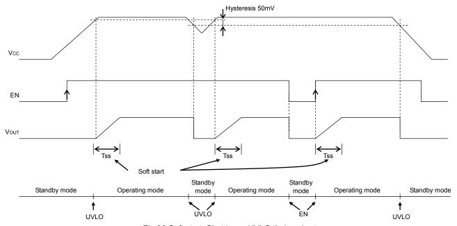
Fig.22 Soft start, Shutdown, UVLO timing chart
