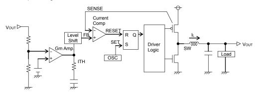
Fig.19 Diagram of current mode PWM control
