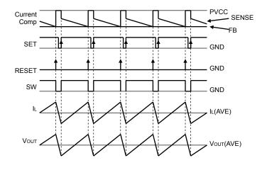
Fig.20 PWM switching timing chart
