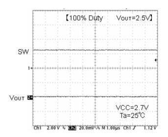
Fig. 16 SW waveform Io=600mA
