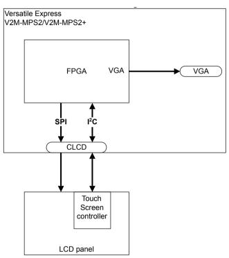
Figure 2-8 VGA and CLCD interfaces.
