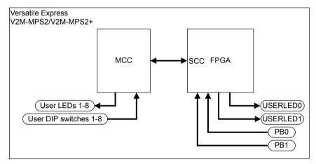
Figure 2-11 Motherboard FPGA and MCC user interface
