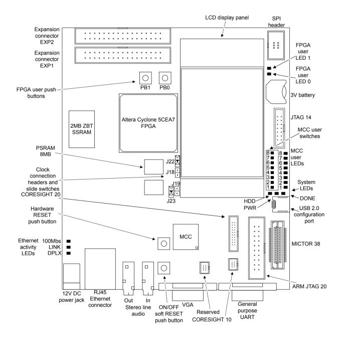
Figure 1-1 Upper face of the V2M-MPS2 motherboard.
