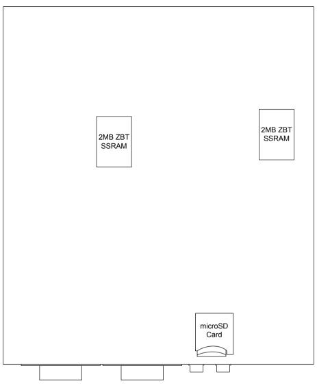
Figure 1-2 Lower face of the V2M-MPS2 motherboard.
