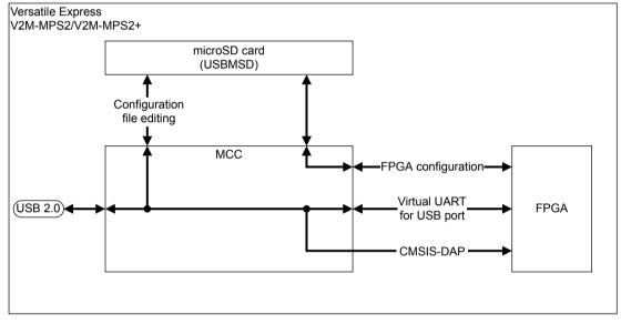
Figure 2-5 Motherboard USB 2.0 Full Speed interface
