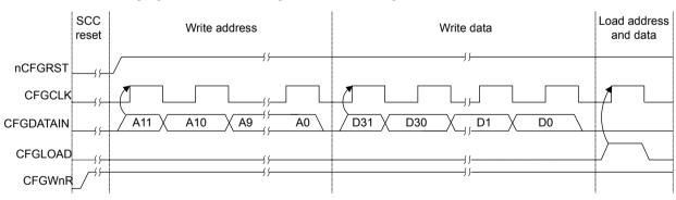
The following figure shows the timings for the WRITE operation.
